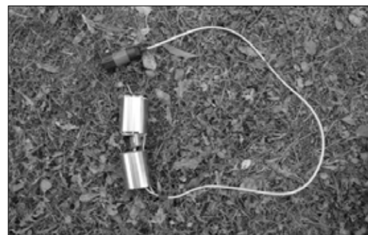
Fig. 2. “Baby EMS 62 modular sap flow system for small stems or branches”.
