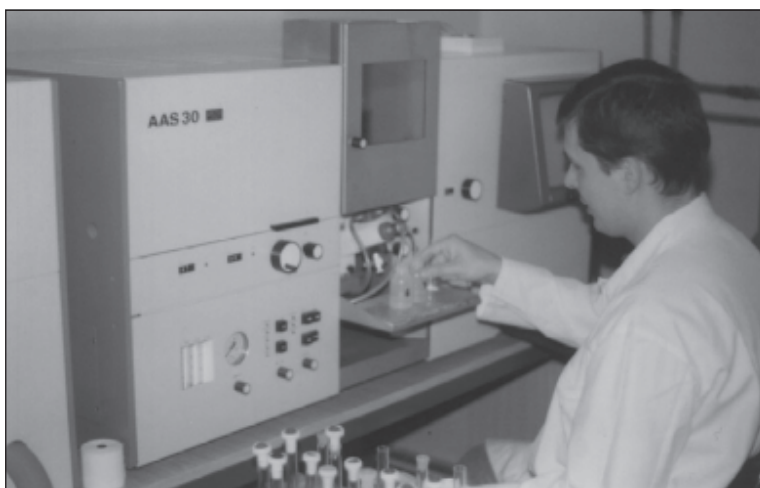
Fig. 1. Determination of basic elements (AAS) in samples of precipitation and throughfall in laboratory of IFE SAS
